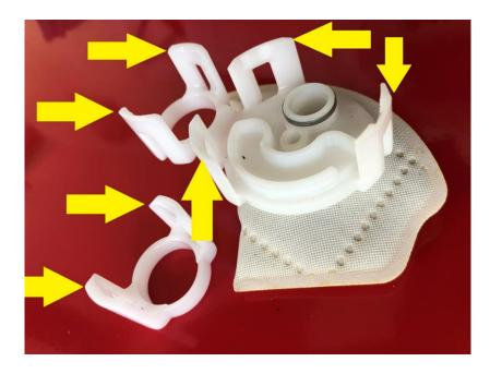
183. Fuel exposure weakens these plastic tabs and clips depleting durability and elasticity.
