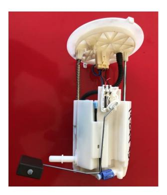
179. As Figure 7 below demonstrates, the fuel pump module drops into the fuel tank through an access hole on the topside of the tank. A retainer ring ensures that the flange and O-ring create a tight seal against the tank surface, preventing fuel escape.
