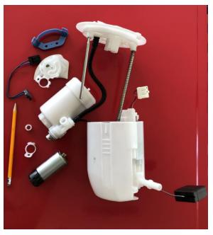
181. The fuel pump module's housing protects the fragile internal components that fit together like puzzle pieces within the module.
